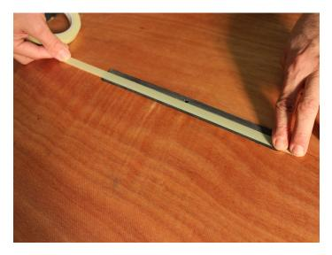
Here, we're varnishing the bottom of the paddleboard, right over the taped-off fin box. At this point, you will have removed the first batch of tape when you cut the fiberglass around the fin box. You will need to re-apply fresh tape before varnishing or painting.
