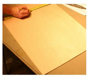
Take two transverse (widthwise) measurements along the back of the aft bottom panel, one measurement at the back edge (above, left), and another about 12" (300mm) forward (above, right). Mark the centers.
