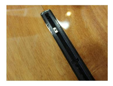
...and rotate the fin down so that the hole aligns with the nut.
