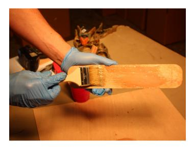
...and glue the cap to the spacer. Use a few small weights to hold the cap in place while the epoxy cures...
