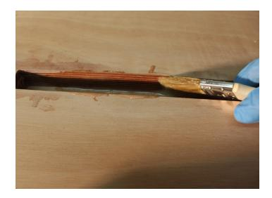
...and coat the exterior of the fin box. Be extra careful not to let any epoxy drip into the fin box channel!
