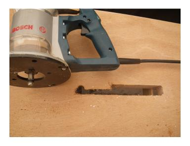
Here's the finished slot, perfectly cut by the router.
