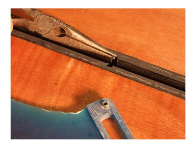
Time to test-fit your fin! The fin pin drops into the center slot, then slides forward or aft along the internal track.
