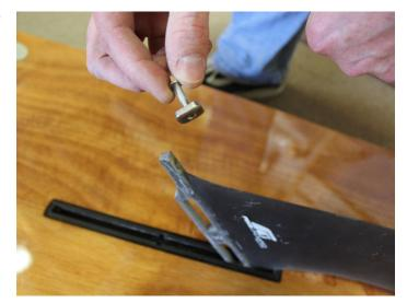
Slide the nut into the groove...
