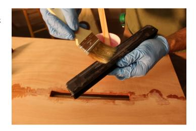
Press the fin box into the slot...
