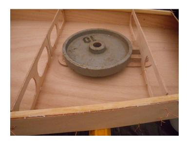
Now it's time to put the first hole in the board! The easiest way to open the slot for the fin box is with a router and a "flush-trim" bit. The bearing of the bit will ride along the inside face of the spacer and the bit will trim a perfect slot. Alternatively, you can use a saber saw or bonsai saw, and sand the edge flush by hand.
