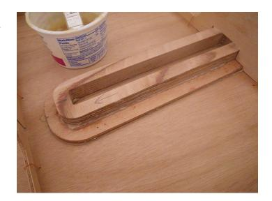
Clean up the excess epoxy from around the baseplate and use a weight to hold the assembly in place while the epoxy cures.
