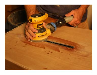
The fin box should be perfectly flush with the surrounding plywood bottom panel.
