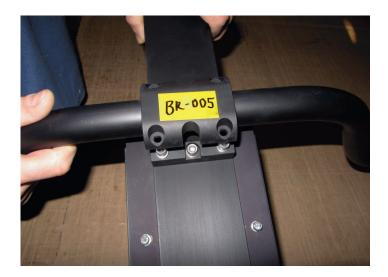
4. Attach the stays to the upright with bolts. The two black nylon washers go between the stay feet and the upright.
