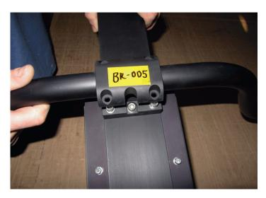
6. Unscrew the track stops and slide the seat on. Ensure the seat is the correct way round: the concave side should face away from the feet.
