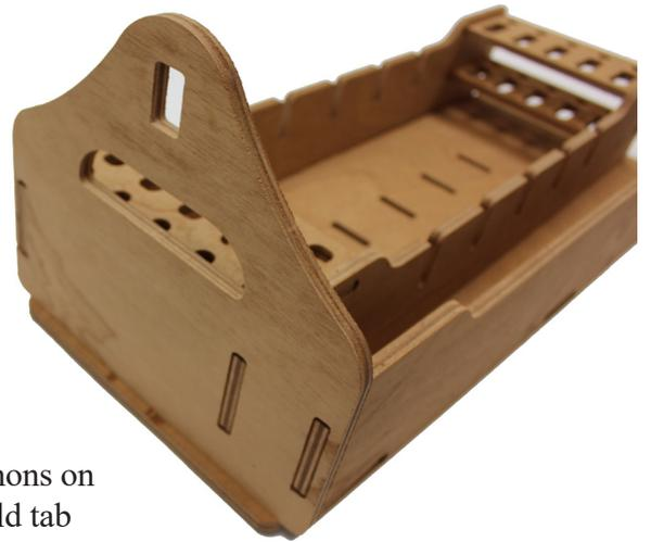
... and rotate them into place. The tenons on the side panels and long divider should tab into the mortises in the end panels.
