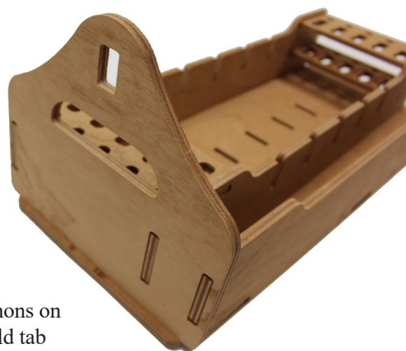
... and rotate them into place. The tenons on the side panels and long divider should tab into the mortises in the end panels.
